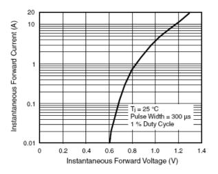
Figure 3. Typical Forward Characteristics Per Diode
