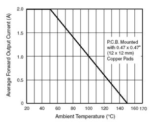
Figure 1. Derating Curve Output Rectified Current
