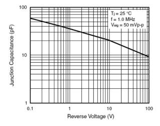
Figure 5. Typical Junction Capacitance Per Diode
